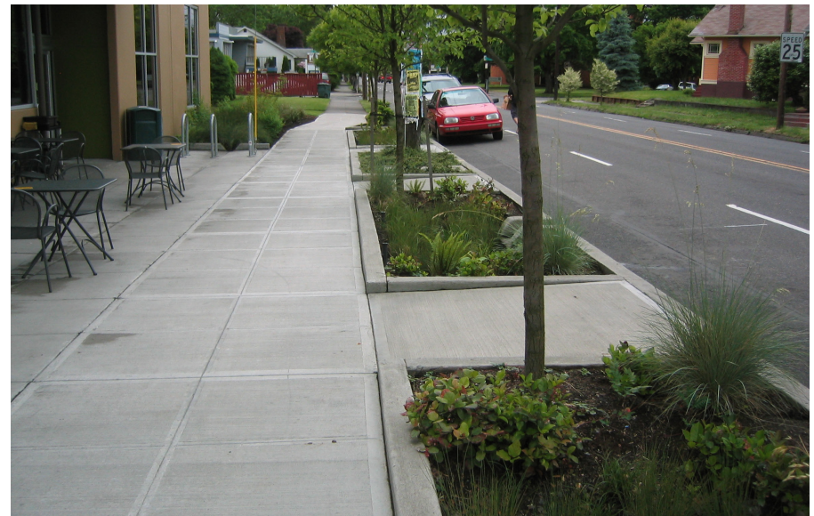
Examples of infiltration and flow-through planters
